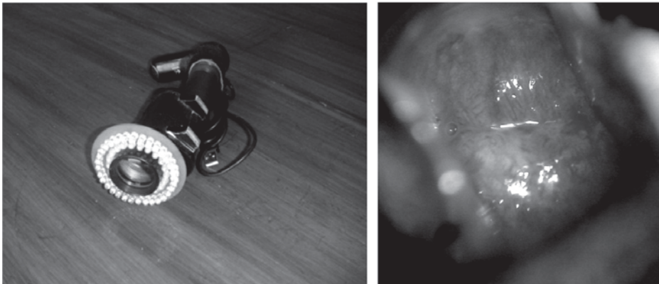
Figure14: Digital microscope (left). A high quality 2MPixel webcam with glass lens was affixed to an ordinary microscope to make a low cost unit. The digital zoom option of the webcam together with selectable magnifications of the microscope makes it very flexible (right image). Still images are captured in JPG format while wmv format is used to save moving images including sound.
