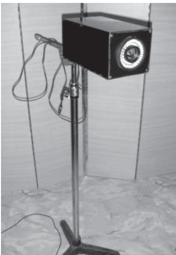
Figure15: Digital Colposcope (left) to detect cervical cancer, produced at a fraction of the cost of commercial devices. A colposcope needs to focus and magnify an object at a distance of about 300mm which is not allowed by standard microscopes or telescopes. This unit was improvised from one part of an ordinary binocular telescope (top left) by changing the length between the eye piece and the objective lenses. Again the high quality webcam as used for the microscope gave a picture quality only available with very expensive colposcopes. A photograph of a cervix taken using this device shows the blood vessels clearly (right).
