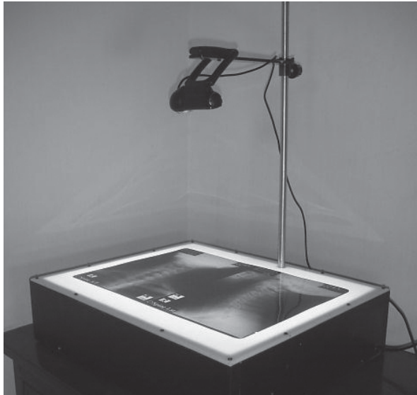
Figure16: Digital X-ray Viewbox (left) and image produced on a computer monitor (right). Multiple white LEDs were used to illuminate the white plastic backing. A high quality webcam was mounted on a stand with adjustable height.
