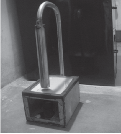
Figure 21: X-ray film optical density measuring instrument developed by the author's group. The X-ray film images is to be placed under the light source, which is within the tube. The light detector and amplifier are inside the box.
